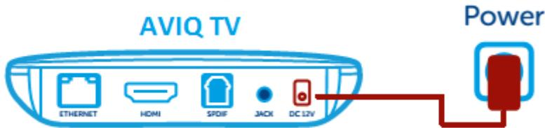
Connect the AC adapter to the STB, then insert the power plug into your wall socket. The STB will immediately turn on when power is connected.
