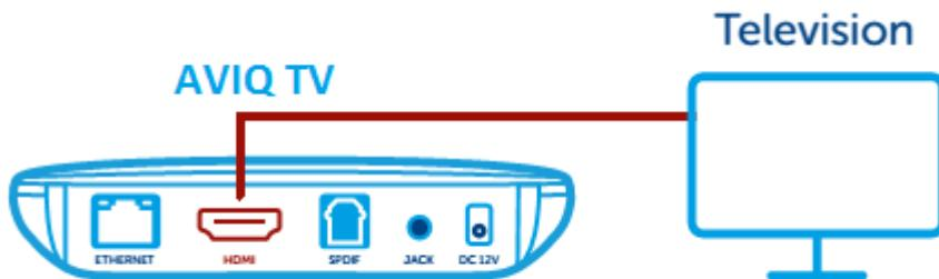
Connect one side of the HDMI cable to your STB, and the other side to your TV. If your TV has multiple available HDMI inputs, please set your TV accordingly. Note that the HDMI cable carries both audio and video signals directly to your TV. If your TV has no HDMI input, you will need to use a SCART adapter.
