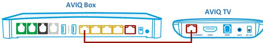
You can connect your TV decoder to your modem/router with a network cable (recommended for better TV service stability) or use WI-FI (see the “Network configuration” section for further details). If you are using the network cable, plug it into the Ethernet port located on the back of your TV decoder and to one of the Ethernet ports of your modem/router (these are generally yellow and marked “Ethernet” or “LAN”).
